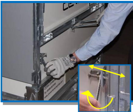
5. The Side panels are unlocked by releasing the 2 latches, the Side is then "eased" in at the bottom to clear the cleats, and then lowered flat
