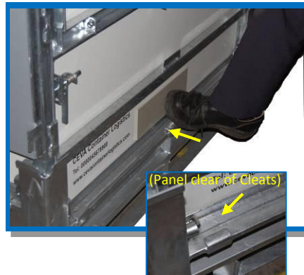
5. The Side panels are unlocked by releasing the 2 latches, the Side is then "eased" in at the bottom to clear the cleats, and then lowered flat
