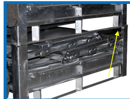
14. By removing the back tilt, the FLT driver has now securely located all four corners of the upper Autoflow 3 onto the lower unit.
