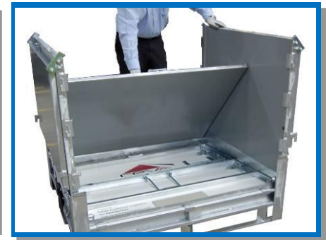
4. The Drop Side Door should be closed. Fold "UP" and Lift over the two notches in the frame. The Latches should now be locked and closed flat
