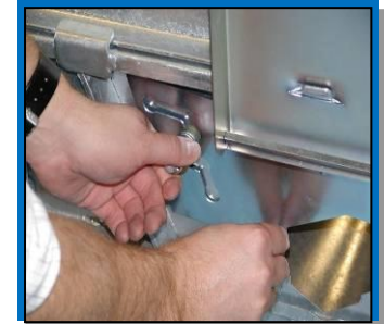
9. Adjust slides to required width setting for the liner in use.
