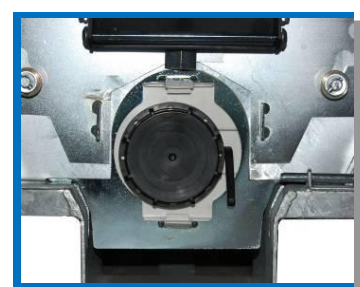
14. The Autoflow 3 / Liner system may be secured from tampering by attaching a seal to the BD Door Lock.. The unit is ready for filling with product
