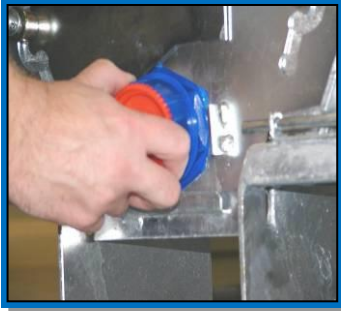
10. Pull through discharge gland and secure into place.
