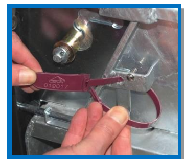
14. The Autoflow 3 / Liner system may be secured from tampering by attaching a seal to the BD Door Lock.. The unit is ready for filling with product
