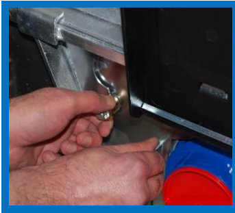
11. Adjust slides to lock the discharge Valve/Gland into place. Push the Gland face hard to ensure it is fitted and will not move during filling.
