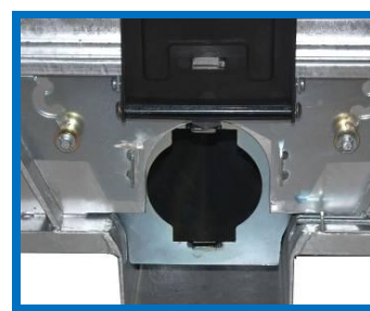
18. This is the cassette used to support the DN50 Valve system.
