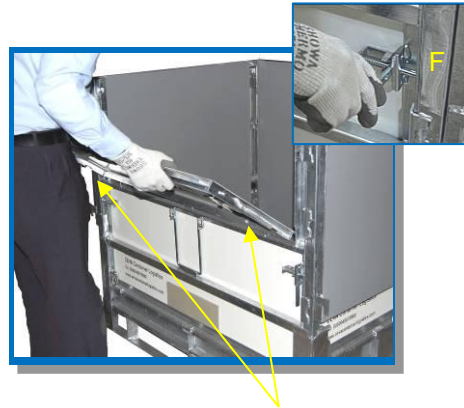
3. Unlock both Lock bolts (F), lift and release drop down panel (G) for easy insertion or removal of liquid liner.
